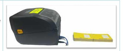
Open the printer lid and feed the Sticker stock through the opening in the back of the Sticker printer.
