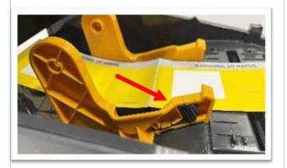
Pull the end of the Sticker as close to the edge of the front of the printer as possible and close the lid.
